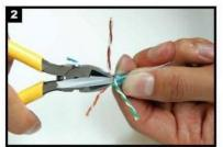
Paarfolie entfernen. Remove pair shielding.
