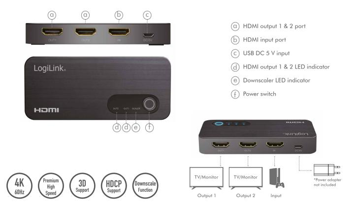
The "Downscaler" function allows the product to display the 4K input resolution on two screens/monitors with different maximum resolutions (e.g. 1080p and 4K) simultaneously. This is useful, for example, when using an older Full HD (1080p) monitor and a newer Ultra HD (4K) monitor at the same time.
