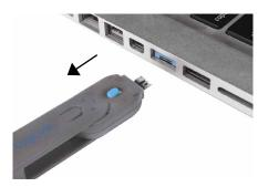
Push the button backwards and pull out the Key. The USB port is locked.
