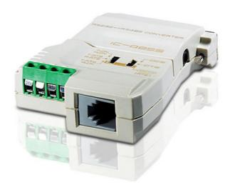
IC485S is a 2-way converter for converting RS-232 signals to and from RS-422/RS-485 signals in long-distance applications up to 1200 m (4000 ft.). It supports the connection of up to 32 hubs and features monitoring to confirm the data passing between devices.
