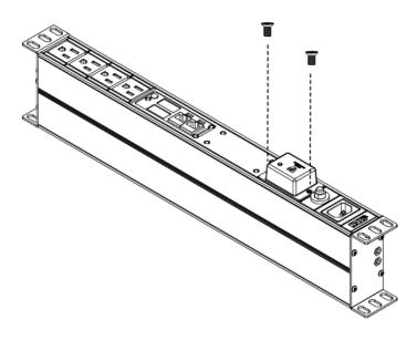
2. Screw the surge protection module into the PDU unit using the two screws you unscrewed in step 1.
