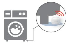
Place under washing machine. Activate alarm when water leakage is detected!
