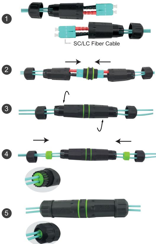
Pass the two cables through the end covers and the long tubes respectively.
