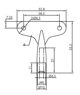
Cable stripper: easily remove the sheathing from the coaxial cable.
